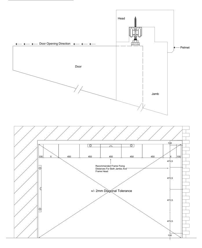
NOTE: This hardware system is designed to be "Top Hung": Therefore the weight of the doors will be carried by the Head Fix Aluminium Track. As such it is necessary to ensure that there are secure fixings through the Frame Head into the partition/ ceiling above. Failure to do so may result in the Frame Head bowing which will adversely affect the functioning of the hardware system.
