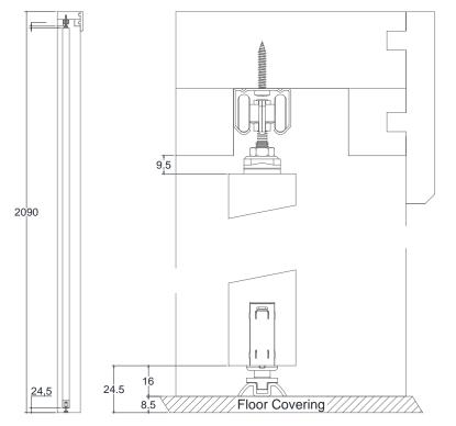
Full length jambs allow for a maximum 8.5mm floor covering: Reduce Jamb length if they are to be installed on top of an existing floor covering
